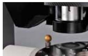
Light sectioning sensor calibration
